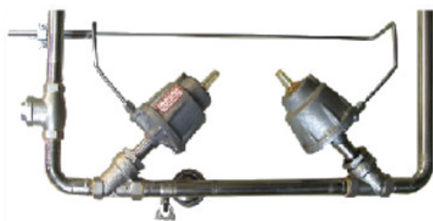
Pipeline system adopts stainless steel sanitary pipe and world brand pneumatic valve
